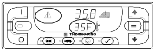
Figure 26: Alarm Icon and Setpoint
