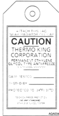
Figure 5: Antifreeze Caution (Attached near radiator fill cap.)
