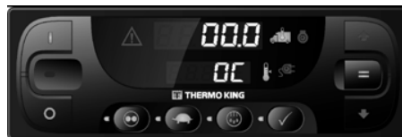
Standard HMI Control Panel
